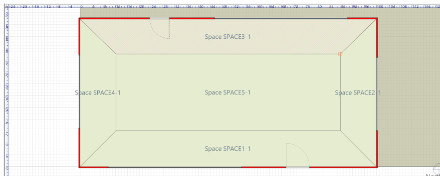
Figure 2.1: SPACE3-1 is the north facing exterior zone of the building.
