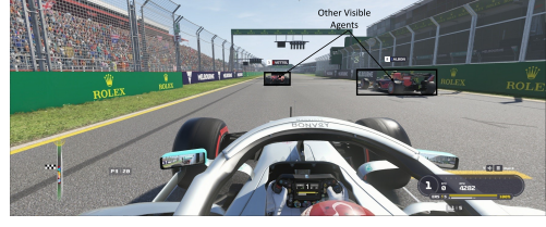
Fig. 2: An example calibration image. The goal is to fit a camera model that can project 3D points in the ego coordinate system to their corresponding pixel location in the F1 game’s output image.
