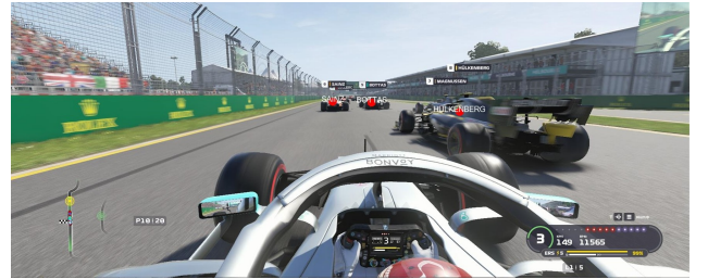
Fig. 3: After model fitting, we can map 3D points in the ego vehicle’s coordinate system to 2D pixel locations in the game images
