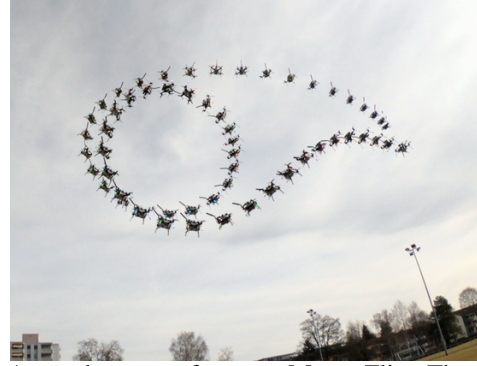
Fig. 3: A quadrotor performs a Matty Flip. The drone is controlled by a deep sensorimotor policy, and uses only onboard sensing and computation.
