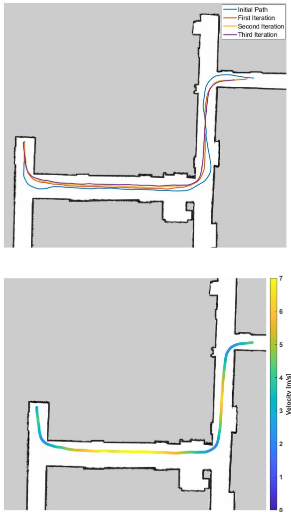
Fig. 6: Iterative approach to generate trajectory over Clemson Fluor Daniel Basement Map
